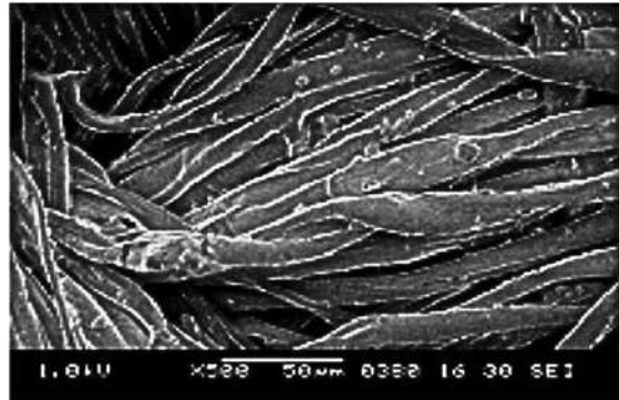
SEM photographs of microcapsule-treated fabric
